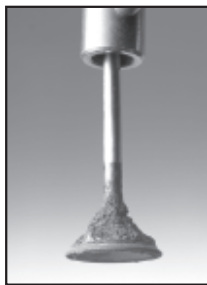
Dirty Intake Valve
