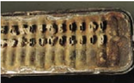
Deposit Restricted Cooling System
